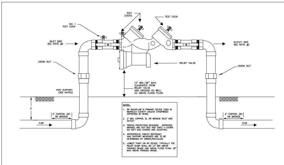
TYPICAL REDUCED PRESSURE PRINCIPLE ASSEMBLY
